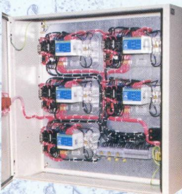
These units incorporate an individual starter and electronic DC brake module for each motor, this ensures that the stand still detection is fully operational and that DC injection is only applied to running motors when the stop button is pushed. The starters are designed for wall mounting and incorporate terminals for connection to remote start/stop buttons on the machine.
